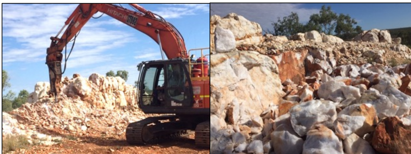
Figure 4.1. Mobile rock-breaker during the 2016 bulk-sampling at Reef 2, May Downs project (left) and some of the stockpiled “clean” quartz (foreground right).
