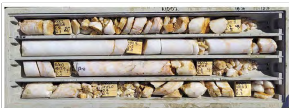
Figure 8-9. Drillhole R2002 from 10.4 – 13.3 m showing a portion of the quartz reef intersection.
